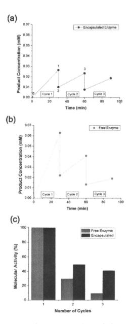
Figure 9. Concentrations of nitrophenol product at the beginning and end of three reaction cycles for (a) encapsulated AP and (b) free AP. The solid lines were drawn to guide the eyes. (c) Relative enzymatic activity of encapsulated and free forms with reaction cycle. Enzyme loading was calculated by measuring the enzyme concentration of the supernatant, after dis-assembly of the AP-NACs. Initial enzyme amount: 0.48 U (0.07 mg)
