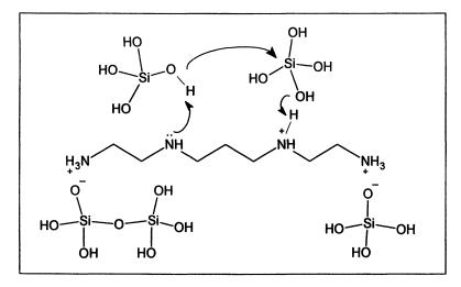
Figure 1. Polyamine-catalyzed silicate condensation is driven by the electrostatic interaction between silicate and cationic amines, combined with acid/base catalysis.
