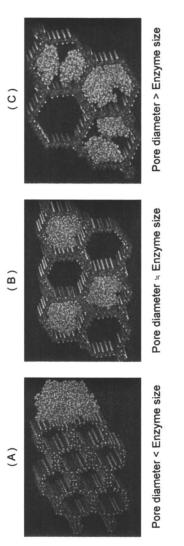
Figure 4. Image models of immobilized enzymes in mesoporous materials with various pore sizes. A: the pore diameter is much smaller than enzyme size, B; the pore diameter is nearly the same size of enzyme molecule C; the pore diameter is much larger than enzyme size
