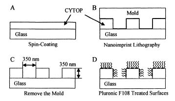
Figure 12. Patterned structures produced by nanoimprint lithography (29): A. spin-coat a layer of CYTOP on glass; B. nanoimprint lithography; C. the resulting structure after removing the mold; D. non-fouling modification of CYTOP surfaces after Pluronic treatment.
