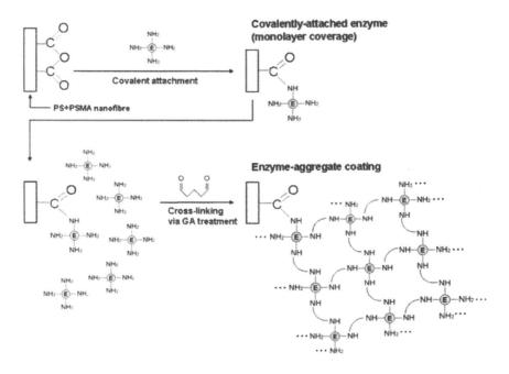
Figure 7. Schematic representation of enzyme-coating on the surface of polymer nanofibers. (Reproduced with permission from reference 10. Copyright 2005 Institute of Physics Publishing.)
