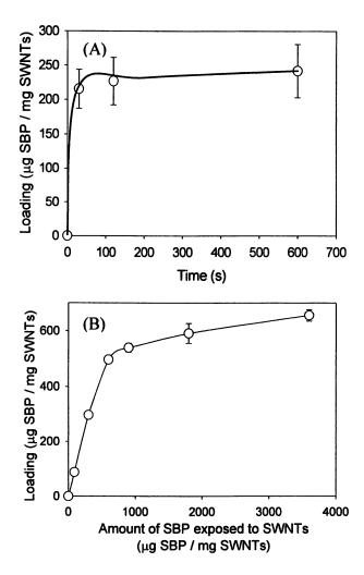
Figure 1. Loading of SBP on SWNTs: (A) Enzyme loading on SWNTs as a function of time using a SBP solution of concentration 0.25 mg/mL. (B) Enzyme loading as a function of amount of SBP exposed to the SWNTs. Error bars indicate the standard deviation of triplicate measurements.
