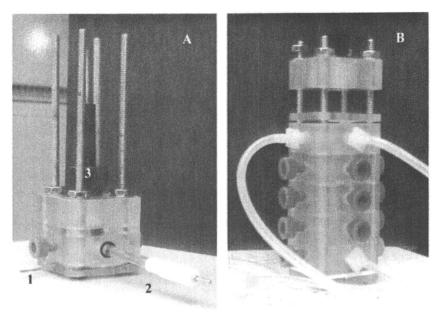
Figure 17. Modular stack cell. In image (A), (1) the platinum counter electrode, (2) reference electrode, and (3) working electrode.
