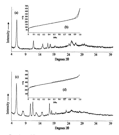
Figure 3 X-ray diffraction patterns and  $N_2$  adsorption isotherms for (a. -b.) as-synthesized 2-D metal organic framework and (c. -d.) the 3-D MOF.
