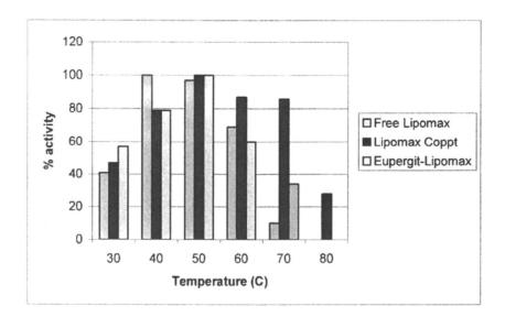
Figure 4. Thermal activity of a LIPOMAX<sup>TM</sup> silica coprecipitate as compared to the soluble enzyme and that immobilized on to EUPERGIT  $C^{\text{®}}$  resin.
