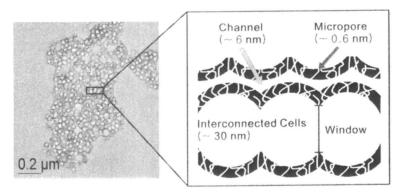
Figure 1. TEM image (left) and schematic illustration (right) of MSU-F-C showing the morphology and the sizes of sub-structures.
