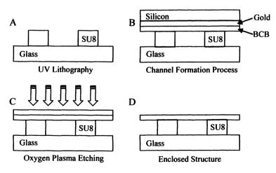
Figure 9. The process of fabricating totally enclosed structures: A. UV lithographically patterned structure; B. The structure is brought in contact with a layer of BCB coated on Au/Si; C. After peeling off the silicon wafer, oxygen plasma etching is used to remove the Au layer; D. The final enclosed structure.
