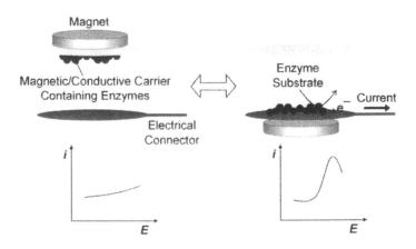
Figure 2. Principle of the magnetically switchable electrochemical biosensing. Expected voltammetric results are depicted schematically for switched off (left) and on (right) states.
