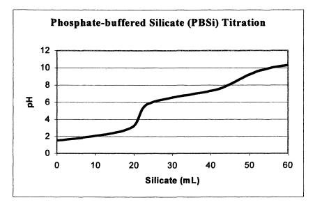
Figure 3. Titration of phosphoric acid (60 mL of 166mM) with sodium silicate (620mM silica) produces phosphate-buffered silicate (PBSi) solutions.
