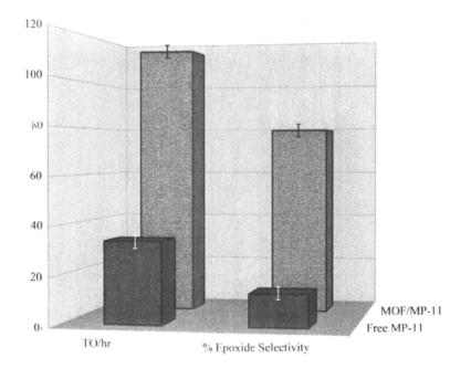
Figure 12. Turnovers per hour and percent epoxide selectivity for the free and immobilized MP-11 during the RT oxidation of α-methylstyrene
