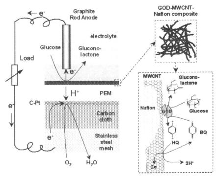
Figure 3. Configuration of GOx-O<sub>2</sub> biofuel cell. PEM: proton exchange membrane (Nafion<sup>®</sup> 117); C-Pt: carbon-supported platinum, cathode catalyst; BQ: benzoquinone; HQ: hydroquinone.
