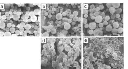
Figure 3. SEM images of AP-NACs with enzyme loadings of (a) 0 wt%, (b) 16 wt%, (c) 18 wt%, and 9 wt%.
