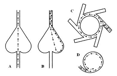
Figure 3. Structures to regulate gliding direction: A. filaments moving upwards are unaffected in their direction of motion; B. Filaments going downwards are redirected upwards (22,23); C. a ratchet pattern used to obtain counterclockwise motion (24,25); D. a structure that can concentrate gliding filaments (25).
