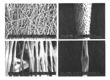
Figure 3. SEM images of PS-PSMA nanofibers produced by electrospinning of a toluene solution of PS-PSMA. (Reproduced with permission from reference 10. Copyright 2005 Institutute of Physics Publishing.)
