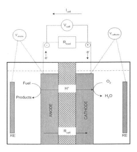
Figure 1. Schematic of an enzyme catalyzed bio-fuel cell.
