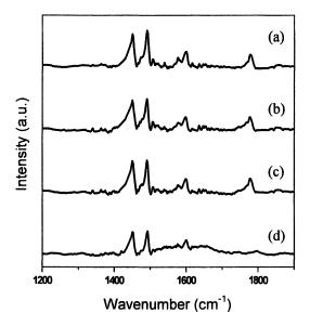
Figure 11. Infrared spectra of PS-PSMA nanofibers after various treatments. (a) as-spun nanofibers, (b) nanofibes washed with phosphate buffer, (c) nanofibers pre-treated with alcohol solution, and (d) nanofibers after alcohol pretrements and reaction with n-propylamine.
