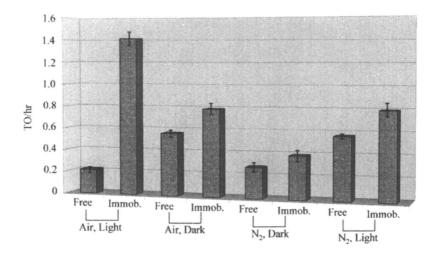
Figure 10. Turnovers per hour for the oxidation of methylene blue catalyzed by free and immobilized MP-11 under air or  $N_2$  and ambient light or dark.
