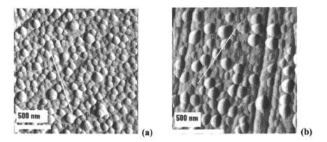
Figure 1. AFM images of (a) 500 loaded Ferrihydrite particles and (b) 2000 loaded ferrihydrite particles deposited on a ZnSe ATR-FTIR crystal.
