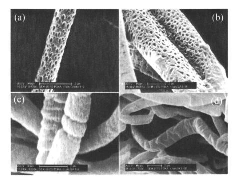
Figure 8. SEM images of (a) CA-CT nanofiber and (b,c,d) EC-CT nanofibers.
