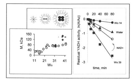
Figure 3. YADH in ternary AOT-water-octane system; Left bottom – molecular masses of protein found by sedimentation analysis; Left upper – schematic representation of the results of sedimentation analysis; Right - time dependence of the residual activity (ln(A/Ao)) of YADH in water and AOT- water- octane system at Wo 14 and 39, pH 8.6, 25°C. Arrow – the stability changes in the presence of NAD<sup>+</sup>
