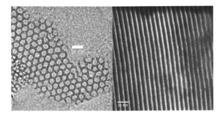
Figure 1. TEM images showing (A) the hexagonal pore structure and (B) the channels in SBA type materials.
