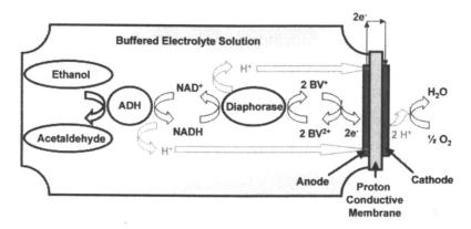
Figure 5. A schematic showing an ethanol enzymatic bio-fuel cell concept based on a similar system proposed by Palmore et al. [23]
