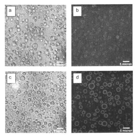
Figure 2. (a,c) Brightfield and (b,d) confocal microscopy images of (a,b) AP-PLLcit aggregates and (c,d) AP-NACs. [PLL]<sub>final</sub> = 0.13 mg/ml; [cit]<sub>final</sub> = 2.1 mM; [SiO<sub>2</sub> NP]<sub>final</sub> = 7.9 wt.%; [AP]<sub>final</sub> = 0.26 mg/ml. PLL was conjugated to FITC.
