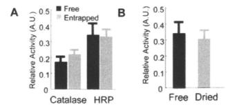
Figure 3. Catalase and HRP are active and stabilized when encapsulated in R5templated silica. Catalase and HRP were encapsulated in R5-templated silica and assayed for activity before drying (panel A) and after drying and rehydrating catalase (panel B). The free catalase control (never dried) is shown in panel B for comparison of activity. (Reproduced with permission from reference 23. Copyright 1998.)
