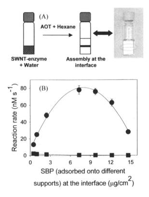
Figure 5. Interfacial assembly of SWNT-enzyme at the aqueous-organic interface.
