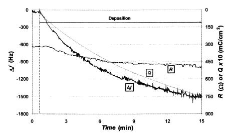
Figure 14. Quartz crystal microbalance result recorded in situ during a potentiostatic polypyrrole film deposition in aqueous solution. Correlation with charge is shown.
