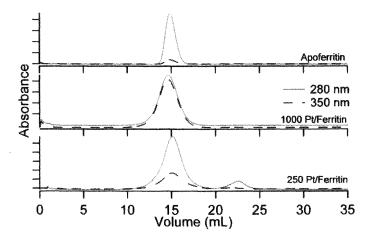
Figure 2. Size exclusion chromatography of ferritin. (A) Unmineralized ferritin,
