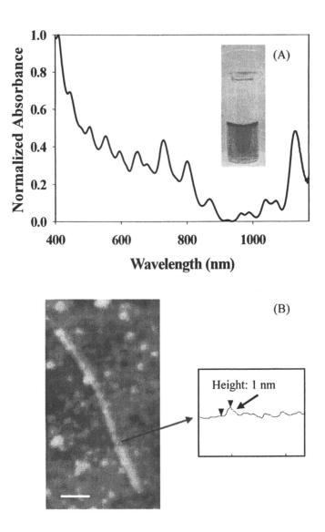
Figure 4. Characterization of solutions of SWNTs obtained using BSA (SWNT-BSA). (A) UV-Vis absorption spectrum of SWNT-BSA. Inset shows a photograph of an SWNT-BSA solution. (B) AFM micrograph of SWNT-BSA. The scale bar represents 100 nm. Line scan shown in the box reveals that the diameter of the SWNT is 1 nm. This figure is adapted from Karajanagi et al. (30).
