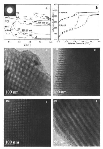
Figure 12. a) SAXS patterns of mesoporous polymer FDU-16 and mesoporous carbon C-FDU-16. The inset is the 2D SAXS pattern of FDU-16. b) N<sub>2</sub> adsorption isotherms of FDU-16 and C-FDU-16. c) and d) TEM images of FDU-16 recorded along [100] and [110] directions. e) and f) TEM images of C-FDU-16 viewed along the same directions. Reproduced from reference 85. Copyright 2005, Wiley.
