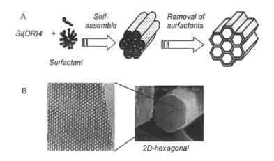
Figure 2. Typical synthesis procedure and structure of mesoporous materials. Silica molecules are self assembled on the surface of micelles and mesoporous materials are obtained after removal of the surfactant.
