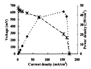
Figure 4. Performance of biofuel cell using composite coated glassy carbon anode. Dashed line: voltage; Dotted line: power density.
