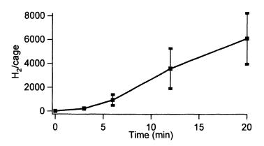
Figure 8.  $H_2$  production from 250 Pt/Ferritin in 0.2 mM Ru(bpy)<sub>3</sub><sup>2+</sup>, 0.5 mM methyl viologen, 200 mM EDTA, and 500 mM acetic acid pH 5.0. **250** Pt/ferritin 3.3 x 10<sup>-10</sup> moles Pt.
