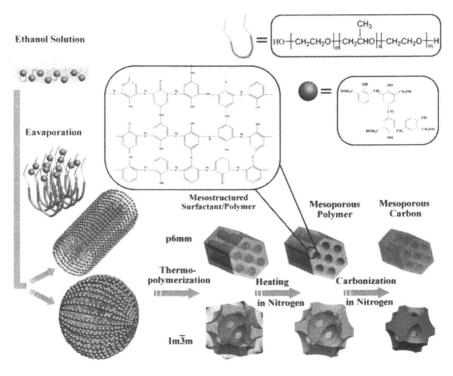
Figure 11. Schematic diagram of the synthetic procedure for mesoporous polymer and homologous carbon frameworks. Adapted from Meng et al. (85) Copyright 2005, Wiley.
