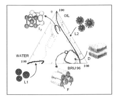
Figure 1. Phase diagram of ternary system Brij 96-water-oil and schematic representation of normal and reverse micelles  $(L_1 \text{ and } L_2)$ , lamellar (D), reverse hexagonal (F) and cubic  $(I_2)$  phases
