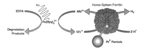
Figure 6. Schematic of the light mediated  $H_2$  production from Pt-Fn. Methyl viologen ( $MV^{2^+}$ ) is used as an electron transfer mediator between the  $Ru(bpy)_3^{2^+}$  photocatalyst and the Pt-Fn responsible for  $H_2$  production.
