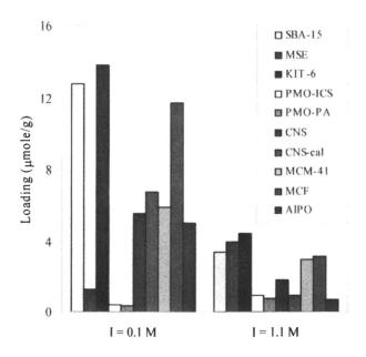
Figure 4. Effect of ionic strength (1) on the amount of cytochrome c adsorbed on to MPS, as determined using a 96 well plate format.
