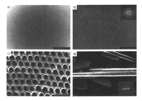
Figure 9. Electron microscopy images of the carbon film. a) Z-contrast image of the large-scale homogeneous carbon film in a 4H3 mm area. The scale bar is 1 mm. b) Z-contrast image showing details of the highly ordered carbon mesostructure. Inset b is the Fourier transform (FT) of the image. The scale bar is 300 nm. c) High-resolution SEM image of the surface of the carbon film. The
