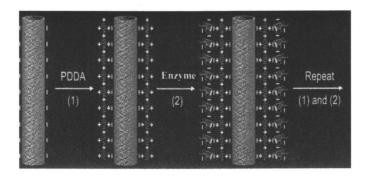
Figure 1. Schematic illustration of the procedure for the attachment of enzymes on a carbon nanotube surface through LBL technique
