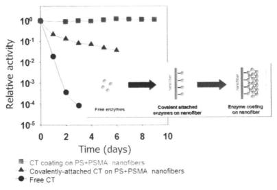
Figure 3. Comparison of stability of a-chymotrypsin (CT) coating nanofibers, covalently attached chymotrypsin on the nanofibers and free enzyme. Adapted with permission from Ref [17]. Copyright 2005 IOP Publishing Ltd.
