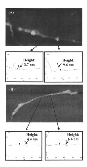
Figure 2. AFM images of enzymes adsorbed onto SWNTs: (A) SBP on SWNTs
