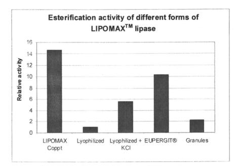
Figure 5. Relative activity of different forms of LIPOMAX<sup>TM</sup> lipase for the esterification of 1-heptanol and oleic acid in isooctane at  $50^{\circ}$ C.
