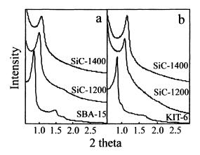
Figure 19. Small-angle XRD patterns of mesoporous silicon carbide replicas and their "parent" mesoporous silica materials with 2D hexagonal (p6m) structure (a) and 3D cubic (Ia 3 d) structure (b). Reproduced from reference 98. Copyright 2006, Wiley.
