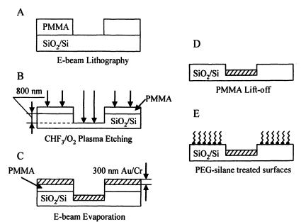
Figure 11. E-beam lithography and plasma etching: A. E-beam lithographily produced structure; B. Oxygen plasma etching to transform the pattern into the  $SiO_2$  layer; C. E-beam evaporation of Au and Cr; D. Lift-off the PMMA layer; E. Non-fouling modification of  $SiO_2$  surface by forming a PEG-silane monolayer.
