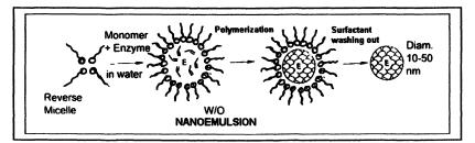
Figure 2. Schematic representation of different manipulations with reverse micelles: 1 - addition of water or/and aqueous solution of enzyme and monomer; 2 - polymerization of the content of an inner cavity; 3 - washing out the surfactant layer resulting in enzyme-containing nanogranules
