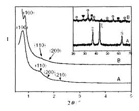
Figure 14. Small-angle XRD patterns of A) NiO and B) Mn<sub>x</sub>O<sub>y</sub> nanowire arrays templated by MWD-SBA-15. Inset: wide-angle XRD patterns of A) NiO nanowire arrays and B) Mn<sub>x</sub>O<sub>y</sub> nanowire arrays (○, ▼, and ■ represent typical diffraction peaks of Mn<sub>2</sub>O<sub>3</sub>, MnO<sub>2</sub>, and Mn<sub>3</sub>O<sub>4</sub> phases, respectively). Reproduced from reference 91. Copyright 2003, Wiley.
