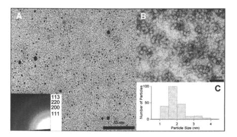
Figure 3. (A) TEM of ferritin 1000 Pt unstained. The inset shows electron diffraction of  $Pt^0$  from ferritin 1000 Pt. (B) TEM of ferritin 1000 Pt stained with 2% uranyl acetate. (C) Histogram of Pt particle diameters in ferritin 1000 Pt. Average  $1.9 \pm 0.8$  nm from 215 particles. Scale bar = 50 nm.
