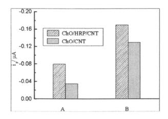
Figure 6. Amperometric responses of two types of enzymes modified GC electrode for choline detection in 0.1 M Tris buffer solution containing 2.0 mM (A) and 9.0 mM (B) choline (pH 8). (Reproduced with permission from reference 18. Copyright 2006.)
