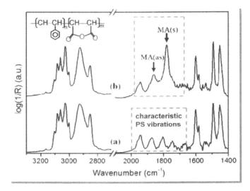
Fgiure 4. Infrared spectra of PS and PS-PSMA nanofibers. The maleic anhydride symmetric and asymmetric vibration peaks are maked with arrows.
