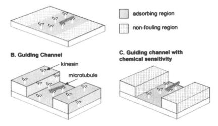
Figure 2. Three basic ways to confine filament motility: A. chemical confinement – motility contrast is obtained by contrast in active surface motor density among surfaces; B. physical confinement – filaments can move on both upper and lower surfaces; C. combined confinement – filaments only move within channels. Reproduced with permission from Nano Lett. 2003, 3, 1651-1655. Copyright 2003 Am. Chem. Soc.
