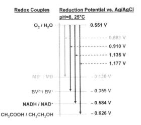
Figure 6. Redox couples in an enzymatic ethanol fuel cell and their reduction potential versus the Ag/AgCl reference electrode at pH 8 and 25°C. (Reproduced with permission from the author. Copyright by held by author.)
