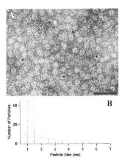
Figure 4. (A) TEM of ferritin 250 Pt stained with 2 % uranyl acetate. (B) Histogram of Pt particle diameters in ferritin 250 Pt. Average  $1.8 \pm 1.2$  nm from 99 particles. Scale bar = 50 nm.
