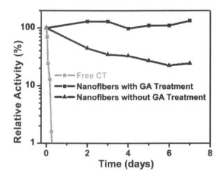
Figure 6. Stability of CT-loaded composite nanofibers treated with and wihtout GA under 250 rpm shaking conditions in phosphate buffer. The deactivation of free CT under the same reaction conditions is also shown for comparison. (Reproduced with permission from reference 11. Copyright 2005 The Royal Society of Chemistry.)
