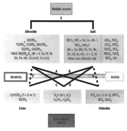
Figure 4. General scheme of the "acid-base pair" concept and guided synthetic routes for mesoporous minerals. Reproduced from reference 59. Copyright 2003, Nature.
