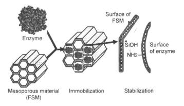
Figure 3. Typical procedure of enzyme stabilization in mesoporous materials.
