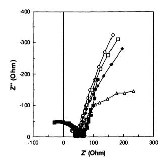
Figure 10. Nyquist plots for the Ni/PGC (O: -0.6 V,  $\Box$ : -0.5 V, and  $\Delta$ : -0.4 V, vs. Ag/AgCl) and SS/PGC ( $\blacksquare$ : -0.5 V and  $\blacklozenge$ : -0.3 V, vs. Ag/AgCl) electrodes with different DC biases. (Reproduced with permission from reference 45. Copyright held by author.)
