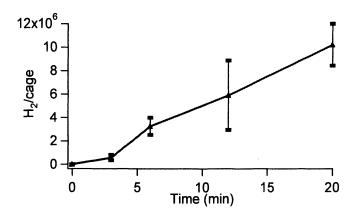
Figure 7.  $H_2$  production from 1000 Pt/Ferritin in 0.2 mM Ru(bpy)<sub>3</sub><sup>2+</sup>, 0.5 mM methyl viologen, 200 mM EDTA, and 500 mM acetic acid pH 5.0.  $\blacksquare$  1000 Pt/ferritin 1.1 x 10<sup>-9</sup> moles Pt.
