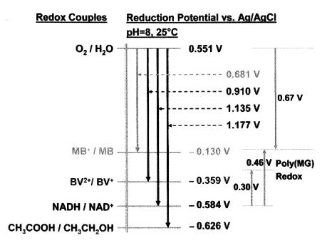
Figure 9. Formal redox potentials for poly-(MG) coated on glassy carbon electrode and the associated  $V_{cell}^{\circ}$ . (Reproduced with permission from the author. Copyright held by the author.)
