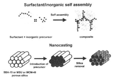
Figure 1. Schematic representation of general pathways leading to mesostructured and mesoporous nonsiliceous materials. Reprinted from reference 46. Copyright 2001, ACS.
