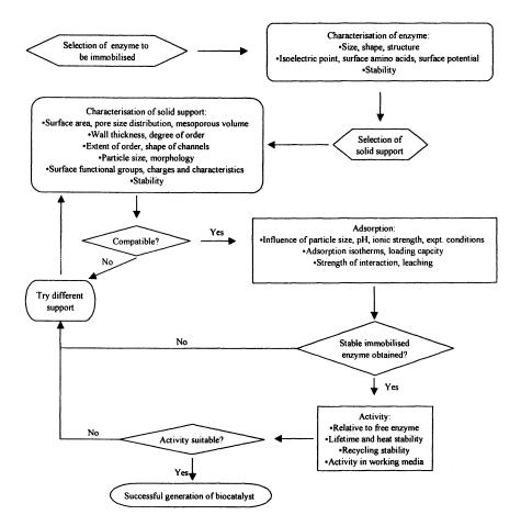
Figure 6. Protocol for the generation of novel immobilised enzyme biocatalysts (18).
