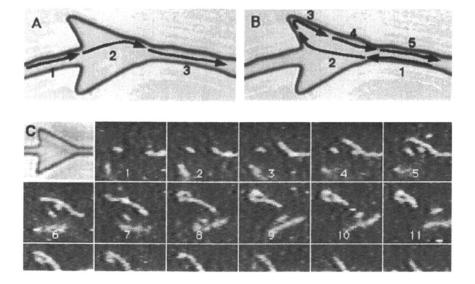
Figure 5. Arrowhead function as a rectifier of microtubule movements in the lithographically patterned channel over kinesin units at the bottom: (A) The scheme shows that a microtubule entering the arrowhead from the correct direction (from the left side entrance) passes through the arrowhead pattern.
