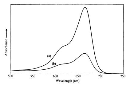
Figure 8. UV-Vis spectra of methylene blue solution a) before and b) after 3 hours of reaction catalyzed by the MOF immobilized MP-11
