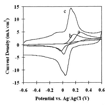
Figure 1. Representative cyclic voltammograms of HQ/BQ redox couple on base glassy carbon (a), Nafion<sup>®</sup>-coated glassy carbon (b) and MWCNT-Nafion<sup>®</sup> coated glassy carbon(c) electrodes. Testing conditions: 0.5 mM HQ in 0.1 M pH 7.0 phosphate buffer, scanning rate: 10 mV/s.
