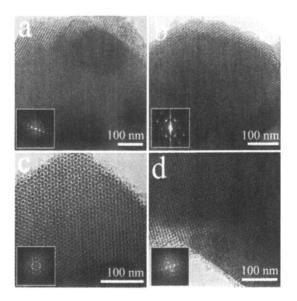
Figure 18. TEM images of mesoporous silicon carbides SiC-SBA15-1200 taken along [110] (a)and [100] (b) directions, and SiC-KIT6-1400 along [111] (c) and [531] (d) directions. Insets show their corresponding Fourier diffractograms. Reproduced from reference 98. Copyright 2006, Wiley.
