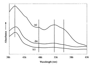
Figure 6. UV-Vis spectra of solid a) MP-11, b) MOF immobilized MP-11, and (c) MOF immobilized MP-11 after oxidation of methylene blue
