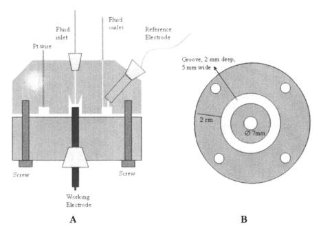
Figure 2. Schematic illustration of (A) a lab-built wall-jet flow cell;(B) bottom scheme of upper piece of wall-jet flow cell.
