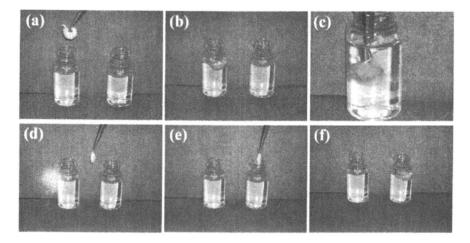
Figure 1. A series of photographs showing a non-woven nanofiber bundle being used in one reaction vial (a, b), recovered with tweezers (c,d), and transferred to another reaction vial (e, f).
