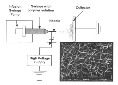
Figure 2. Schematic view of electro-spinning process. Inset shows a scanning electron microscopy (SEM) image of electro-spun polymer nanofibers.
