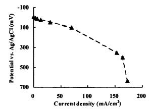
Figure 5. Polarization curve of the anode.
