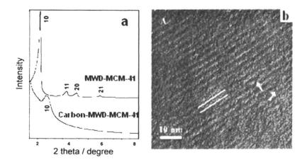
Figure 16. a) XRD patterns of MWD-MCM-41 and its carbon replica, and b) TEM image of carbon nanowires replicated from MWD-MCM-41. Adapted from Tian et al.(90) Copyright 2003, RSC.
