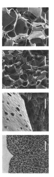
Figure 3. Chitosan scaffolds. Scale bar dimension (L to R): 225 µm, 56.25 µm, 56.25 µm, and 22.5 µm.
