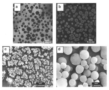
Figure 5. (a) Bright field, (b) confocal, and (c,d) SEM images at two different magnifications of BSA-NACs. [PLL]<sub>final</sub> = 0.13 mg/ml; [cit]<sub>final</sub> = 2.1 mM; [BSA]<sub>final</sub> = 3.1 mg/ml; [SiO<sub>2</sub> NP]<sub>final</sub> = 7.9 wt%. BSA was conjugated to FITC.
