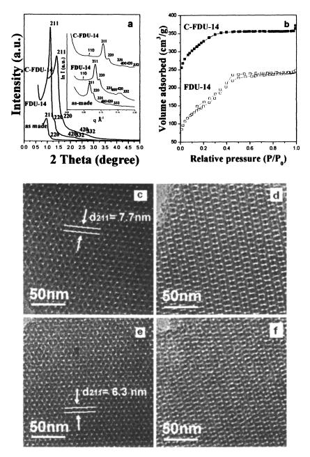
Figure 13. a) XRD and SAXS (inset a) patterns of as-made FDU-14, FDU-14 and C-FDU-14. b) Nitrogen sorption isotherms of FDU-14 and C-FDU-14. c)-f) TEM images of FDU-14 (c, d) and C-FDU-14 (e, f) viewed along [111] (c, e) and [311] (d, f) directions. Adapted from Zhang et al. (86) Copyright 2005, ACS.
