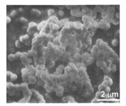
Figure 1. Scanning electron micrograph of R5-templated silica.
