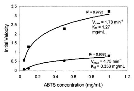
Figure 4. Kinetics of unstirred encapsulated HRP vs. free HRP. The  $V_{max}$  and  $K_M$  values were calculated based on the initial velocity of HRP acting on its substrate, ABTS at increasing concentrations in unstirred systems. Squares represent free enzyme, circles represent encapsulated enzyme.
