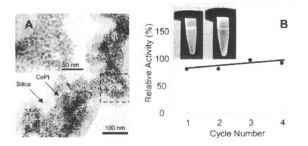
Figure 5. Biomimetic silica encapsulation of magnetic particles and catalase Panel A: TEM micrograph of CoPt nanoparticles encapsulated in biomimetically-templated silica. Panel B: Catalase was co-encapsulated with iron oxide nanoparticles in R5-templated silica and catalase activity was assayed after separating the silica-encapsulation matrix from the solution using a magnetic stand (shown) over several cycles.
