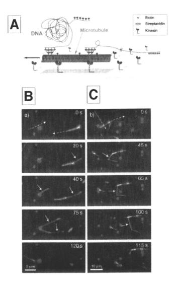
Figure 11. (A) DNA transporting and stretching using microtubules moving over kinesin-functionalized surface in the presence of ATP. (B) Stretching DNA between a surface and one motile microtubule: Two condensed DNA molecules attached to the substrate surface by one of their ends are grasped at their second end by motile microtubules (dark grey, moving in the direction of the dotted white line) and are consequently stretched (light grey; white arrows).
