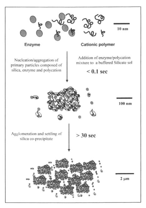
Figure 3. Model of the silica co-precipitation process.
