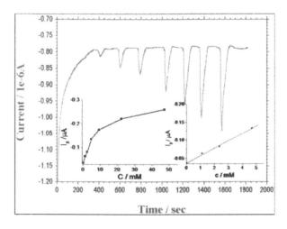
Figure 7. Amperometric response of choline oxidization at a ChO/HRP/CNT/GC electrode by a series of injections of different concentrations of choline solution (from left to right: 0.05 mM, 1.1 mM, 2.4 mM, 5.0 mM, 9.4 mM, 22.4 mM, and 47 mM) in 0.1 M Tris buffer (pH 8). Inset is the plot of peak current vs. choline concentration. (Reproduced with permission from reference 18. Copyright 2006.)
