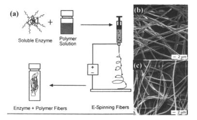
Figure 5. (a) Electrospinning of enzyme-polymer composite nanofibers and (b, c) SEM images of electrospun enzyme-polymer composite nanofibers. (Reproduced with permission from reference 11. Copyright 2005 The Royal Society of Chemistry.)
