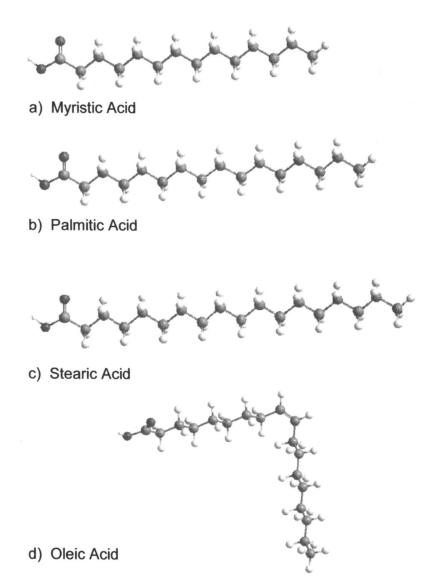
Figure 8. Structure Fatty Acid Components of Soybean Oil
