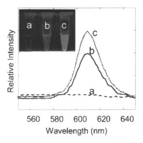
Figure 6. Fluorescence of silica-encapsulated quantum dots. Quantum dots were encapsulated in silica using R5 as a template. Tubes and curves labeled: (a) represent R5-templated silica alone, (b) represent free quantum dots in solution, and (c) represent quantum dots encapsulated in R5-templated silica.
