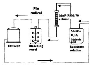
Figure 8. Schematic diagram of the thermally discontinuous immobilized MnP bleaching system.
