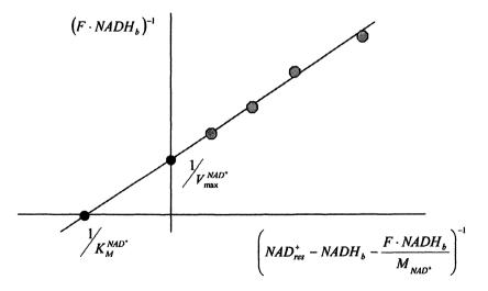
Figure 11. Lineweaver-Burke plot with a lumped mass transfer model [52] for immobilized enzymatic catalytic electrode, which can be used to estimate  $V_{max}$ and  $K_M$  for the specific enzymatic system.
